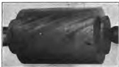
Fig. 137. Gavel Roughed to Shape.
